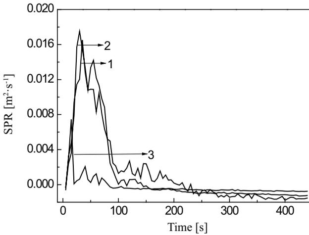
Fig. 7. SPR curves of pure pine needles and flame-retarded pine needles
