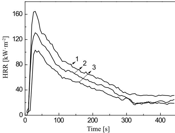
**Fig. 5.** HRR curves of pure pine needles and flame-retarded pine needles
