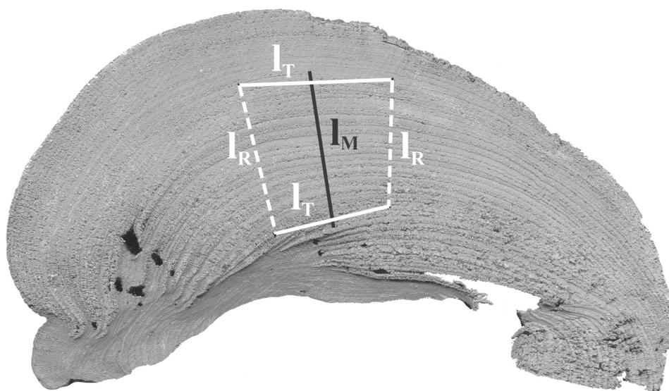
Fig. 2b. A cross-sectional sample of a subfossil log with measured sections marked,  $I_T$  – tangential sections,  $I_R$  – radial sections,  $I_M$  – section for measurements of macroscopic characteristics.
