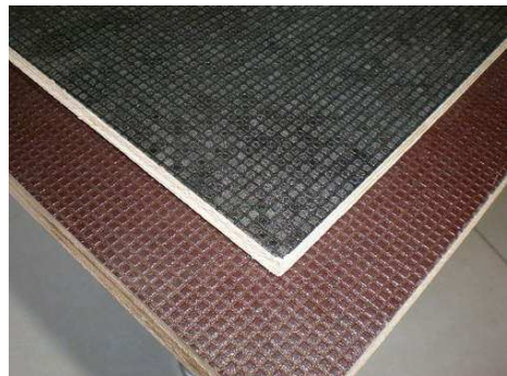
Fig. 1. Left: until WW II the use of solid wood and plywood for car construction was common. Right: birch phenolic film-faced plywood for floors. (Photos by Corrado Cremonini)
