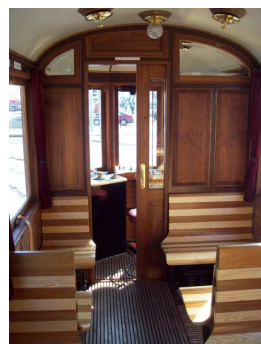
Fig. 2. Left and Right: Plywood and solid wood are a cheap and enduring solution for the floors, walls, ceilings and interior furniture of light-rail public transport. (Photos by Corrado Cremonini)
