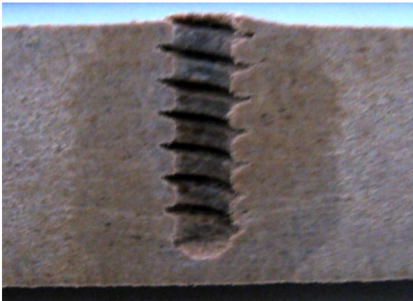
Fig. 4. A cross section of the modified MDF sample by the PUR reinforcing agent (shows the area of modification of the prebored pilot hole for euro screw)
