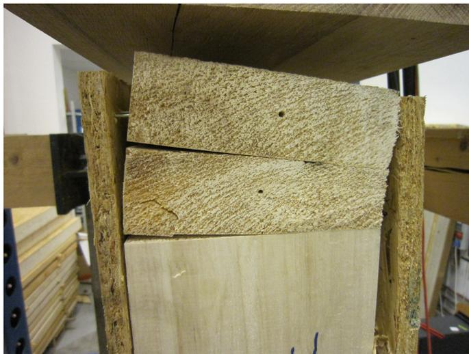
**Fig. 5. Deformation of the upper stud**
