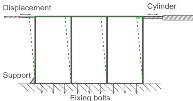
**Fig. 4. Schematic view of the shear test**
