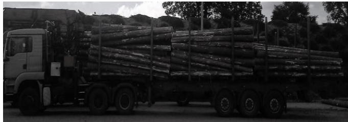
Fig. 6. Transport set truck and semi-trailer with different wood assortments: a) five-axle (3+2) with Ls; b) six-axle with Sw4.4; c) five-axle with Sw8.8; d) six-axle with Sw4.0
