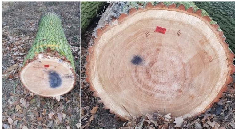
Fig. 2. Visible presence of foreign bodies in wood
