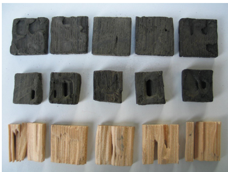
Fig. 1. Condition of wood samples after 4 weeks of feeding by termites: top – heartwood of subfossil Quercus robur from Dołhobrody; center – heartwood of subfossil Quercus robur from Pułtusk; bottom – sapwood of contemporary Pinus sylvestris
