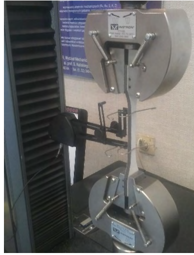
Fig. 2. Specimen in the jaws of an INSTRON 5699 testing machine with extensometer attached
