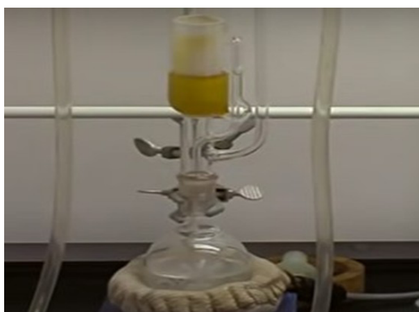
Fig. 2. Determination of extractive content of control and thermally modified specimen using Soxhlet apparatus
