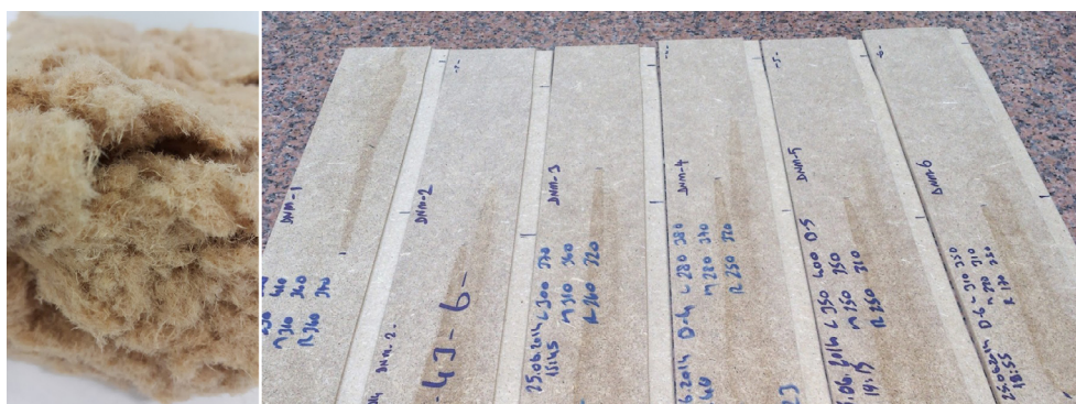
Fig. 1. Fibers (left) and HDF test samples (right)
