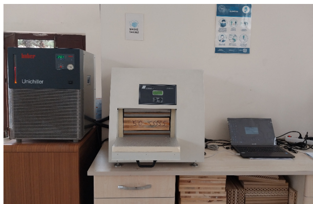
Fig. 4. Device used to determine thermal conductivity coefficients and thermal transmittance coefficients
