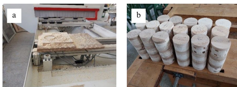
Fig. 5. Preparation of sound absorption test samples: a) processing of test samples on CNC machine, b) sound absorption test samples ready for testing
