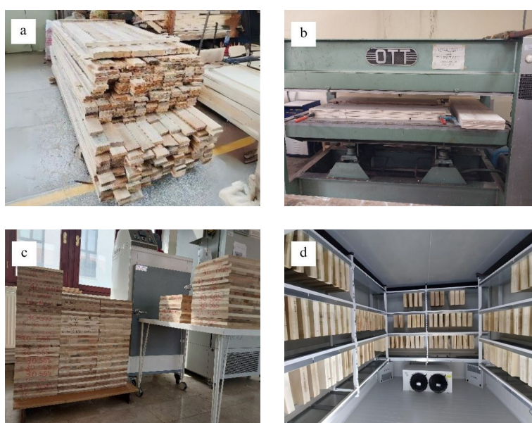
Fig. 1. CLT production: a) solid wood material, b) CLT pressing process, c) dimensioned CLT panels, d) conditioning of test samples
