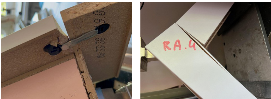
Fig. 8. Damage to door frame samples after tests
