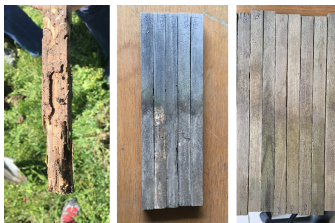
Fig. 3. From left to right: sapwood, heartwood, and impregnated wood
