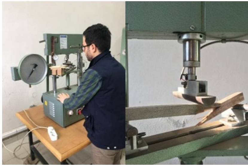
Fig. 1. Determination of bending strength and modulus of elasticity in samples
