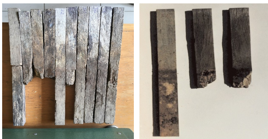
Fig. 4. Unimpregnated beech sapwood test samples from the present study (left). Unimpregnated beech sapwood test samples from a previous study (Zeleniuc et al., 2003)
