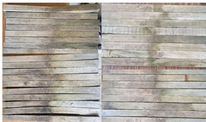
Fig. 5. Images of the above-ground and underground parts of the impregnated samples after three years in soil
