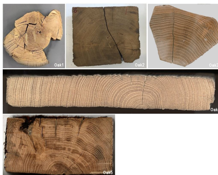
Fig. 1. From upper left: fragment of bog oak taken from the trunk of a tree found in a gravel pit in Kłaj, Lesser Poland (Oak1), fragment of oak construction in bell tower of the Collegiate Basilica of the Holy Spirit in Przeworsk (Oak2), sample of oak from a wooden beam of scaffolding bricked into the wall of St. Nicholas' Church in Gniew (Oak3), fragment of oak structural beam from a granary in Drawsko Pomorskie (Oak4), fragment of beam from the Czaniec water dam in Porąbka (Oak5)
