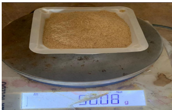
Fig. 1. Milled control sapwood specimen being weighed on a scale before determination of chemical components
