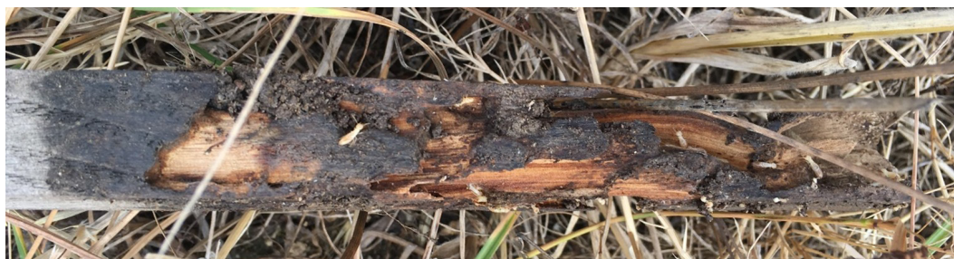
Fig. 3. Termite activity on chestnut samples
