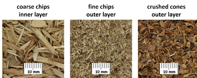
Fig. 1. View of wood chips and shredded pine cones used in the production of the panel
