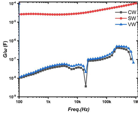
Fig. 5. Frequency-dependent conductance ( $G/\omega$ ) plot for maple
