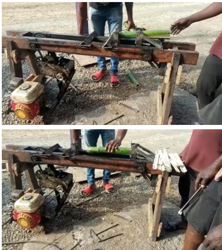
Fig. 8. Prototype of the Mobile Bamboo Culm Splitting Machine during field evaluation with bamboo culms of varying diameters, demonstrating its operational performance
