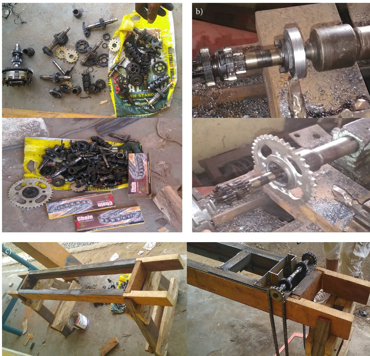
Fig. 4. Stages in the fabrication process of the Mobile Bamboo Culm Splitting Machine (MBCSM). (a) Locally sourced machine parts and components, including chains, sprockets, and gears; (b) machining of shafts for the gear and pulley assembly. (c) Wooden and mild-steel structural frame under construction; assembled frame with chain and gear mechanism mounted
