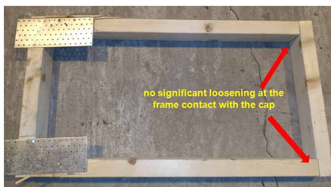
Fig. 13. Element with screwed connection after the study (general view)
