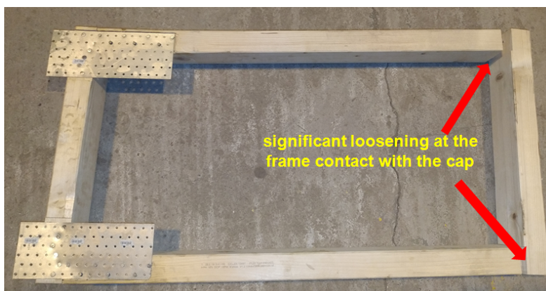
Fig. 10. Element with nailed connections after the study (general view)
