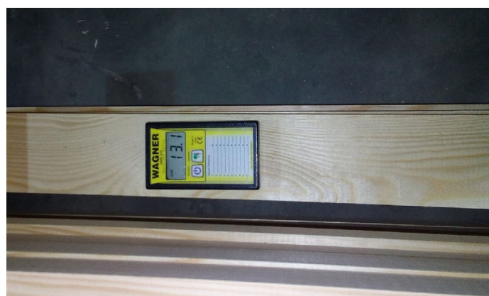
Fig. 2. Moisture measurement of an example beam (BEAMJ1-2)
