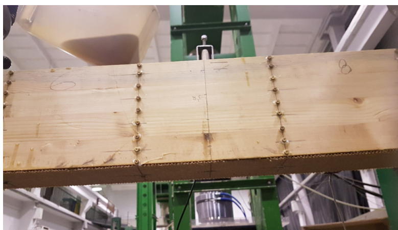
Fig. 3. Reinforcement of glued laminated timber beams with rods and fabrics – final stage
